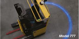
The 777 Arc light is the most recent addition to the warehouse and forklift safety range of products. Creating a half halo, this light is able to cover the entire back side of a forklift with an incredibly intense beam.
