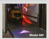
Dot pattern safety lights have become a staple for warehouse and forklift safety over the last several years. The **Model 770** has a very sharp, spot beam where as the **Model 4415** is a bit wider and not as intense. The **Model 4415** also has some unique applications in the agricultural industry in highlighting malfunctioning spray nozzles. The **Model 560** plays an essential role in protecting operators and pedestrians from the potential dangers of moving machinery.
